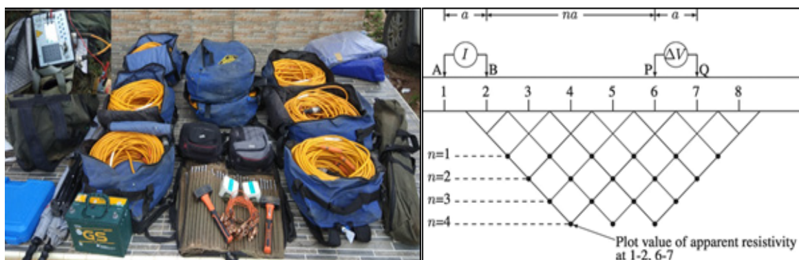
Figure 6. ERT IRIS Instruments (left) and the sequence of dipole-dipole measurement (right)
