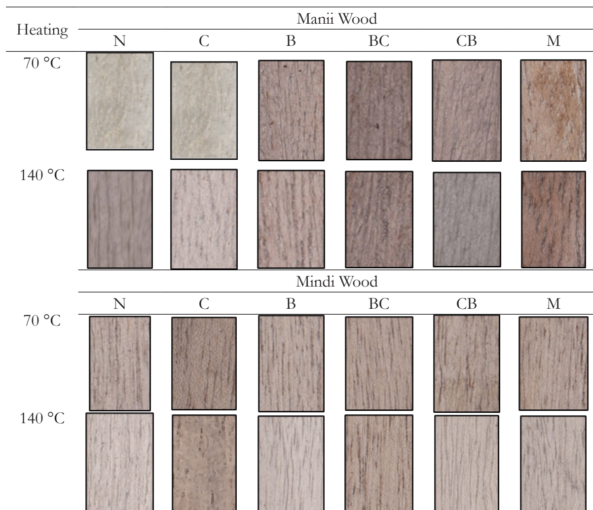
Figure 12. The color changes after weathering of manii and mindi wood treated without impregnation (N), with boric acid (B), chitosan (C), boric acid-chitosan (BC), chitosan-boric acid (CB), mixture combination boric acid +chitosan (M), and heating temperatures (70 °C and 140 °C).
