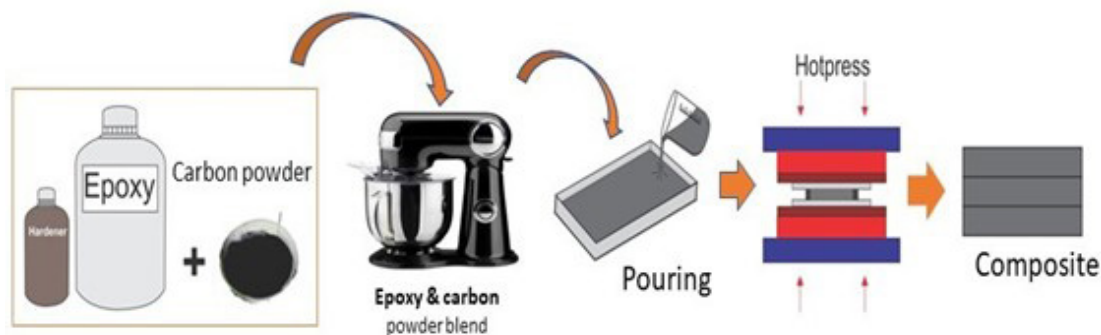
Figure 2. Production of epoxy composites reinforced with carbon powder/ Paederia foetida fiber.
