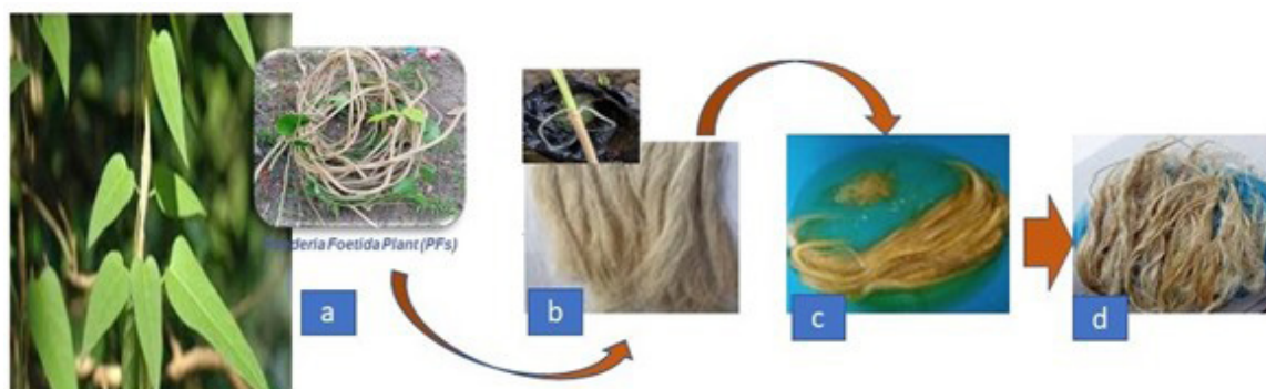
Figure 1. (a) Paederia f. plants, (b) Separation of fibers bundles from the stem (PFs), (cd) NaOH alkaline treatment for 2 h, and (d) Fibers drying
