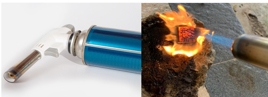
Figure 2. Heating torch (a) and burning test of a wood sample using a heating torch (b)
