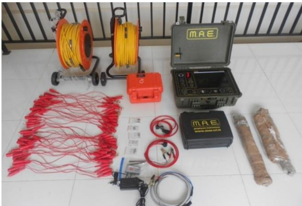
Gambar (Figure) 4. Alat MAE X612-EM VHR Multi-Channel Resistivitymeter (MAE X612-EM VHR Multi-Channel Resistivitymeter Tools)
